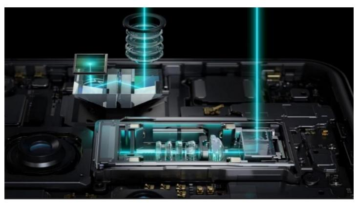
for DSLR-grade zooms to be fitted into a small camera bump without compromising on sensor size or camera quality. The same 3x Triple Prism Design is also implemented on the standard model to reduce the camera module to just 3.01mm for an overall sleek
